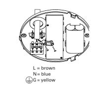
Secure mains cable using cable clip and screws.
