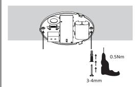
Drill where indicated and use wall plugs and screws, to fix the mounting base in the desired position.
