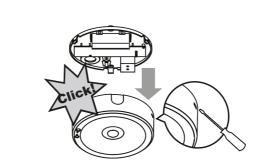
Use screwdriver to press the small hole on the side, then pull up the mounting base.
